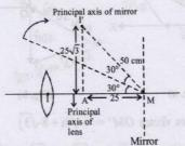
The image formed by convex lens acts as an object for mirror.
